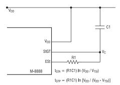
by an external RC time constant driven by ESt. A logic high on ESt causes  $V_C$  (see the Basic Steering Circuit above) to rise as the capacitor discharges. Provided that the signal condition is maintained (ESt remains high) for the validation period ( $t_{\rm GTP}$ ),  $V_C$  reaches the threshold ( $V_{\rm TSI}$ ) of the steering logic to register the tone pair, latching its corresponding 4-bit code (see the Tone Encoding/Decoding on left) into the receive data register.
