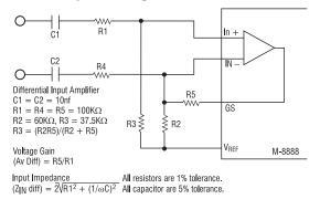
ing the amplifier inputs at  $V_{DD}/2$ . Provisions are made for the connection of a feedback resistor to the op-amp output (GS) for gain adjustment. In a single-ended configuration, the input pins should be connected as shown in the Single-Ended Input Configuration above. Differential Input Configuration above shows the necessary connections for a differential input configuration.
