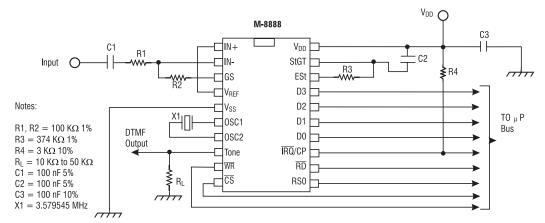
Microprocessor-based systems can inject undesirable noise into the supply rails. M-8888 performance can be optimized by keeping noise on the supply rails to a minimum. The decoupling capacitor (C3) should be connected close to the device and ground loops should be avoided.
