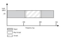
yzed by a microprocessor or counter arrangement to determine the nature of the call progress tone being detected. Frequencies in the reject area will not be detected, and consequently there will be no activity on IRQ/CP as a result of these frequencies.
